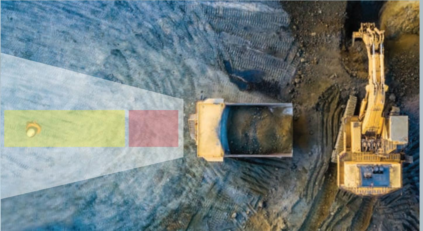
light source and calculates the distance by means of the light reflected from the surface.
